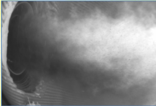
IR picture of pulverized 40 MWth flame. Water-cooled infrared endoscope was used. Dark region indicate low temperature.
